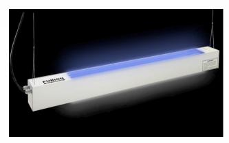
This equipment consists of a matt anodized aluminium profile with matching cover plates. Radiator compartments hold reflectors made of pure polished aluminium. The upward facing compartment holds the UV radiator for ambient disinfection. The downward facing compartment holds the D radiator for room lighting with especially natural light.
